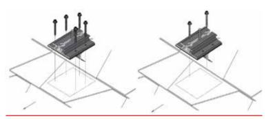
RT-Butyl is Roof Tech<sup>3</sup>s flexible flashing used in one million residential PV systems for the last 27 years. It is the first PV mounting system with Flexible Flashing certified by the ICC. Engineered to withstand wind speeds up to 180 mph and ground snow up to 90 psf.
